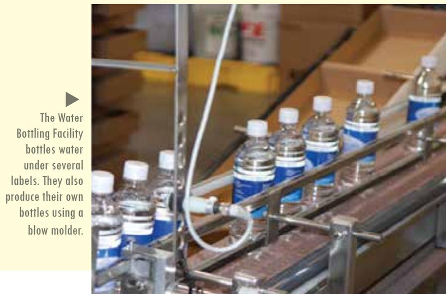
▶ The Water Bottling Facility bottles water under several labels. They also produce their own bottles using a blow molder.
